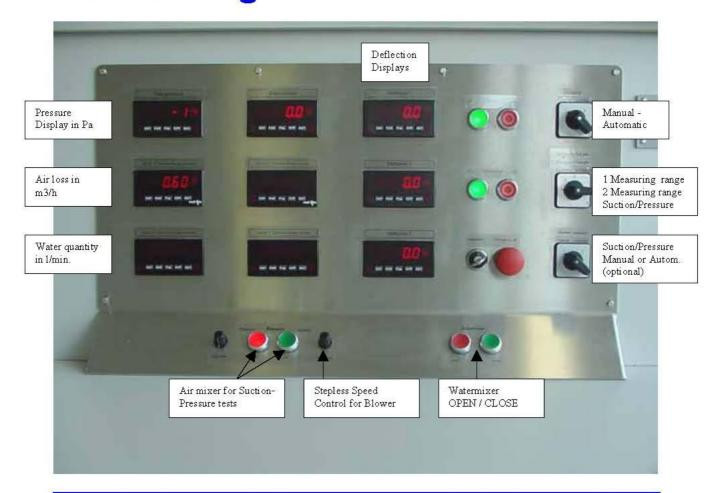
The switch- and control unit **KS MSD Digital** makes it possible to test windows, doors and curtain walls after national and international standards. The operation will be done very convenient and easy from the control desk. All tests can be done very precise through the user. You can read the values **direct** and easy on digital displays.
